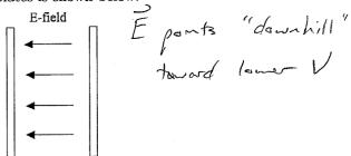
Which plate is at a higher electric potential? (i.e. higher volts)
