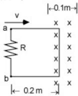
In what direction is the induced current around the loop at the instant shown in the image.
