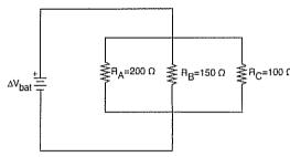
14. Rank the resistors in terms of the current through each resistor.
