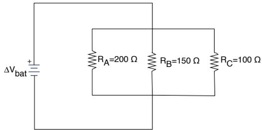
3. Rank the resistors in terms of the current through each resistor.
