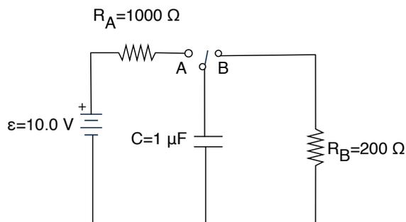
11. What is the maximum charge on each capacitor plate when it is fully charged?
