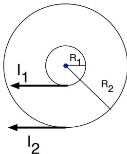
The current in the outer loop is 2 A in the clockwise direction, and its radius is 4 cm. The current in the inner loop is also 2 A in the clockwise direction, and its radius is 1 cm.
