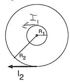
The current in the outer loop is 2 A in the clockwise direction, and its radius is 4 cm.
