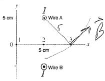
12. Which of these arrows is closest to the magnetic field due to wire A at point 3?
