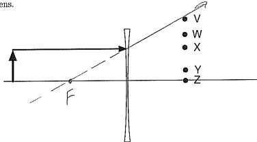
A single ray from the top of the object is drawn in the orientation shown. Through which point will this ray travel?
