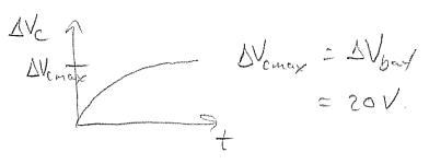
After a very long time, what will be the charge  $(Q_{max})$  on the capacitor?
