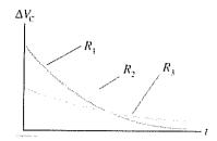
Rank, in order from largest to smallest, the values of the resistances  $R_1$ ,  $R_2$ , and  $R_3$ .
