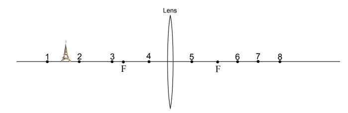
(a) Sketch a ray emanating from the top of the object that is parallel to the optic axis. Show both the incident and refracted rays. Your sketch should be neat and clear.
