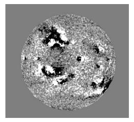
Figure 4: A velocity image from one of the GONG solar telescopes - dark regions correspond to troughs, bright regions to peaks.
