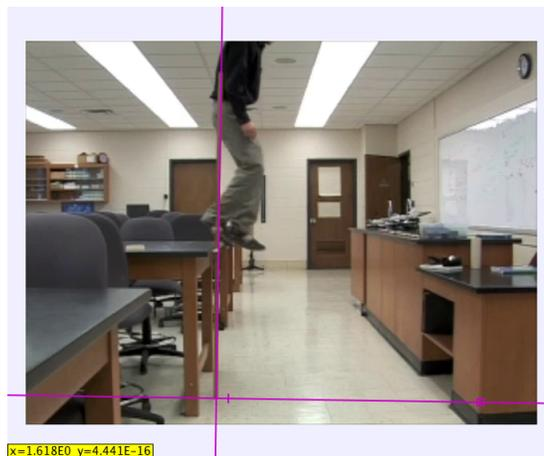
Figure 4: Rotate the coordinate system so that the y-axis is parallel to the 2-m stick.
